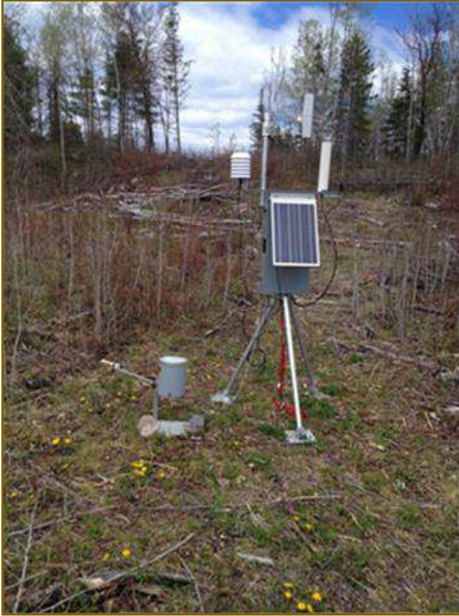
Figure 9 – Superior #2 portable Remote Automated Weather Station (RAWS) located approximately 1/2 mile south of the burn unit.
